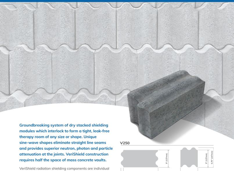
VeriShield radiation shielding components are individual modules combined together to form a composite structure to create the required radiation attenuating environment. The constructed system retains the ability to be deconstructed and reused.
